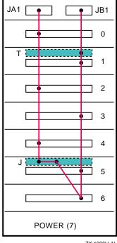
Figure 9-6: BA350 Internal SCSI Bus
